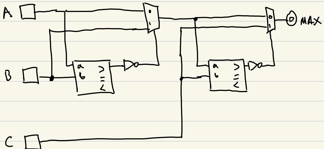
This circuit first selects the maximum value of  $a$  and  $b$ , call it  $\max(a, b)$  then it selects the maximum value of  $\max(a, b)$  and  $c$
